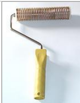
Extra Long 'T' Type Spring Compaction Roller Spring section 17cm x 4cm Ø
