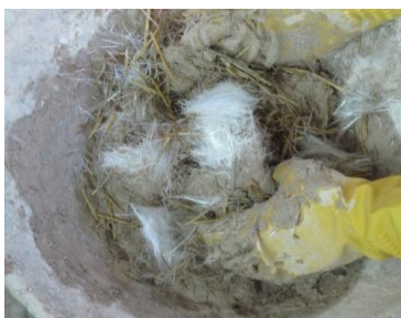
Figure10 - Mixture of glass fibers and traditional mud-straw, photo by author
