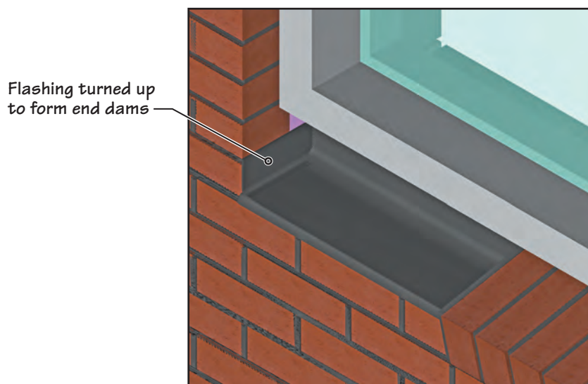
FIGURE 28.10 End dams in flashing, revealed by removing a few bricks of the window sill (in the rowlock course). Weep holes in the brick sill (over the flashing) are not shown for clarity.
