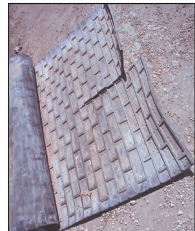
FIGURE 28.47 A rubber template form liner used with thin brick-faced panels.
