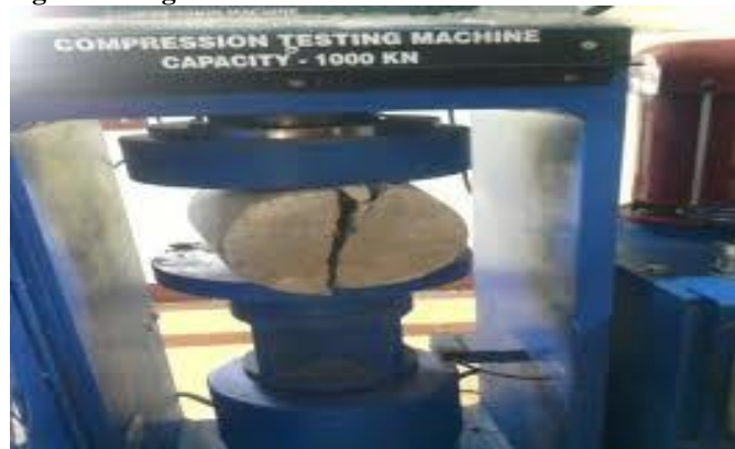
Fig.4. Testing of Cylinders.
