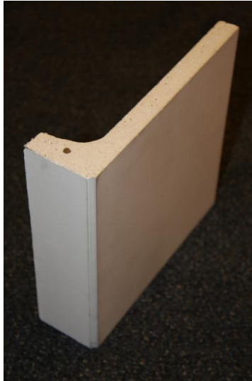
Figure 2 Corner of a GFRC panel with an edge-return, the GFRC panel has been produced with the premixed method
