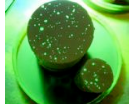
Voids and hollow fibers in the bar appear in ASTM D5117 dye wick testing
