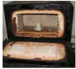
Fiber Content measured by "burn off" of all inorganic constituents of the bar i.e. resin
