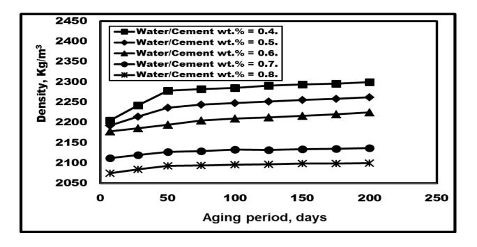
Fig. 8 Effect of W/C weight ratio on the concrete density at different aging periods.
