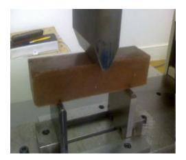
Fig. 2. Flexural test.
