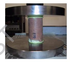
Fig. 4. Compression test.
