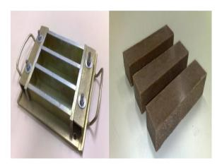
Fig. 1. Flexural and tensile test specimens.
