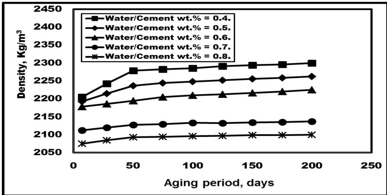
Fig. 8 Effect of W/C weight ratio on the concrete density at different aging periods.
