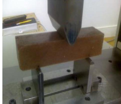
**Fig. 2. Flexural test.**
