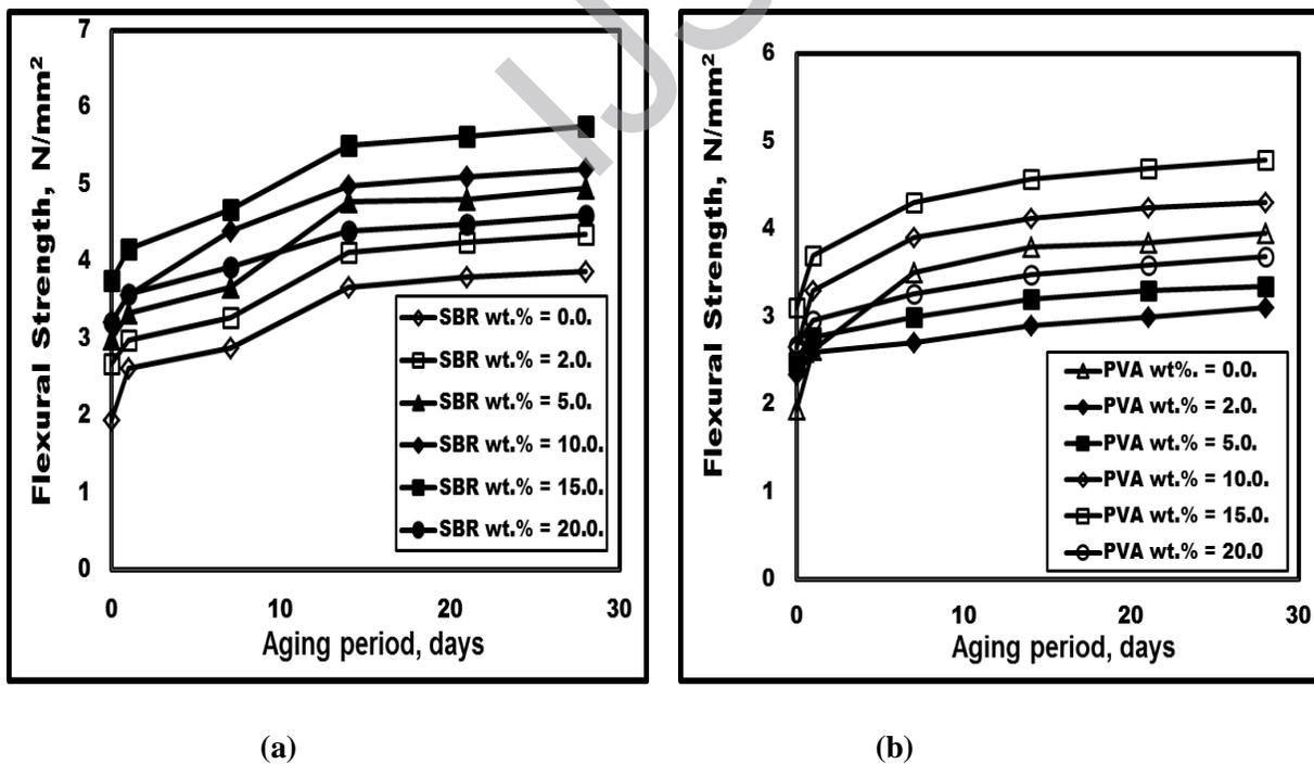
Fig. 7 Effect of SBR and PVA on concrete flexural strength at W/C = 0.46wt.%
