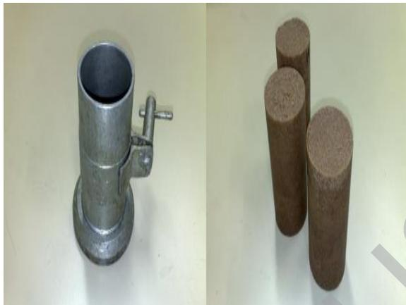
**Fig. 3. Compression test specimen.**
