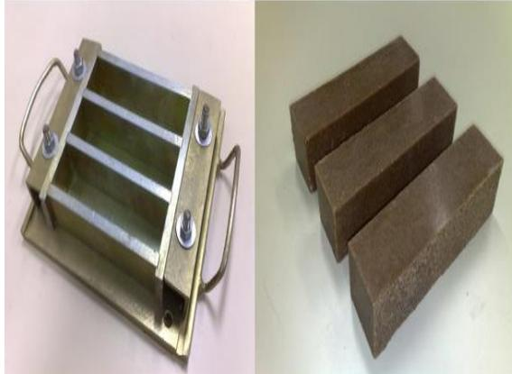
**Fig. 1. Flexural and tensile test specimens.**
