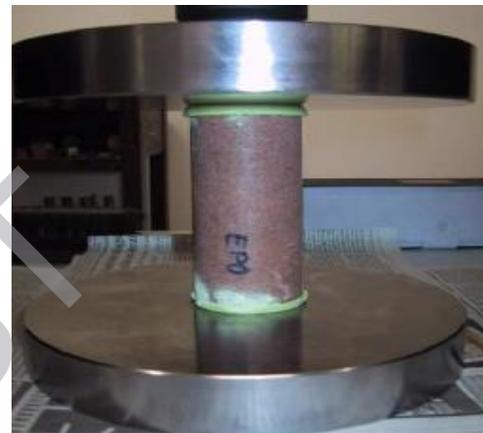
**Fig. 4. Compression test.**
